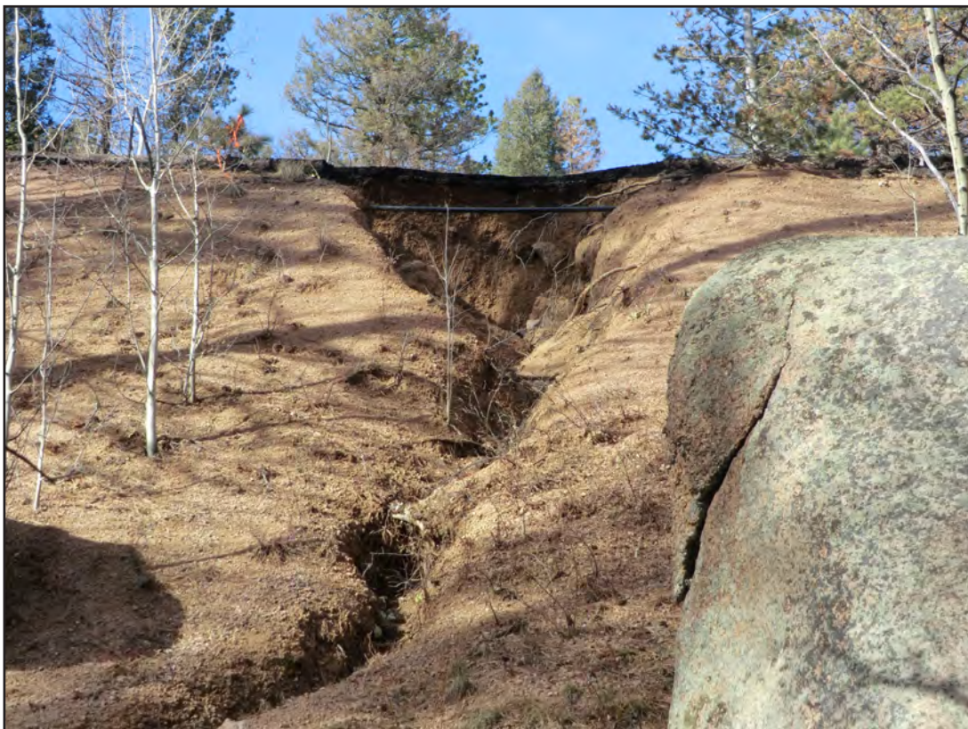
Figure 26. Headcut from poor drainage causing excess erosion below road.
