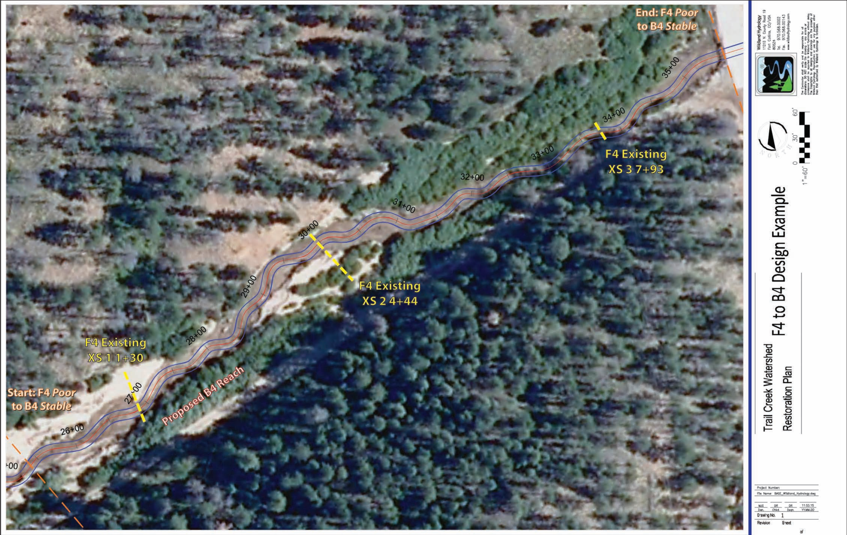
Figure 17. Plan view of the proposed conversion of the F4 to B4 stream type from the West Creek road upstream 1,000 ft to proposed station 25+40, including the existing F4 cross-section locations.
