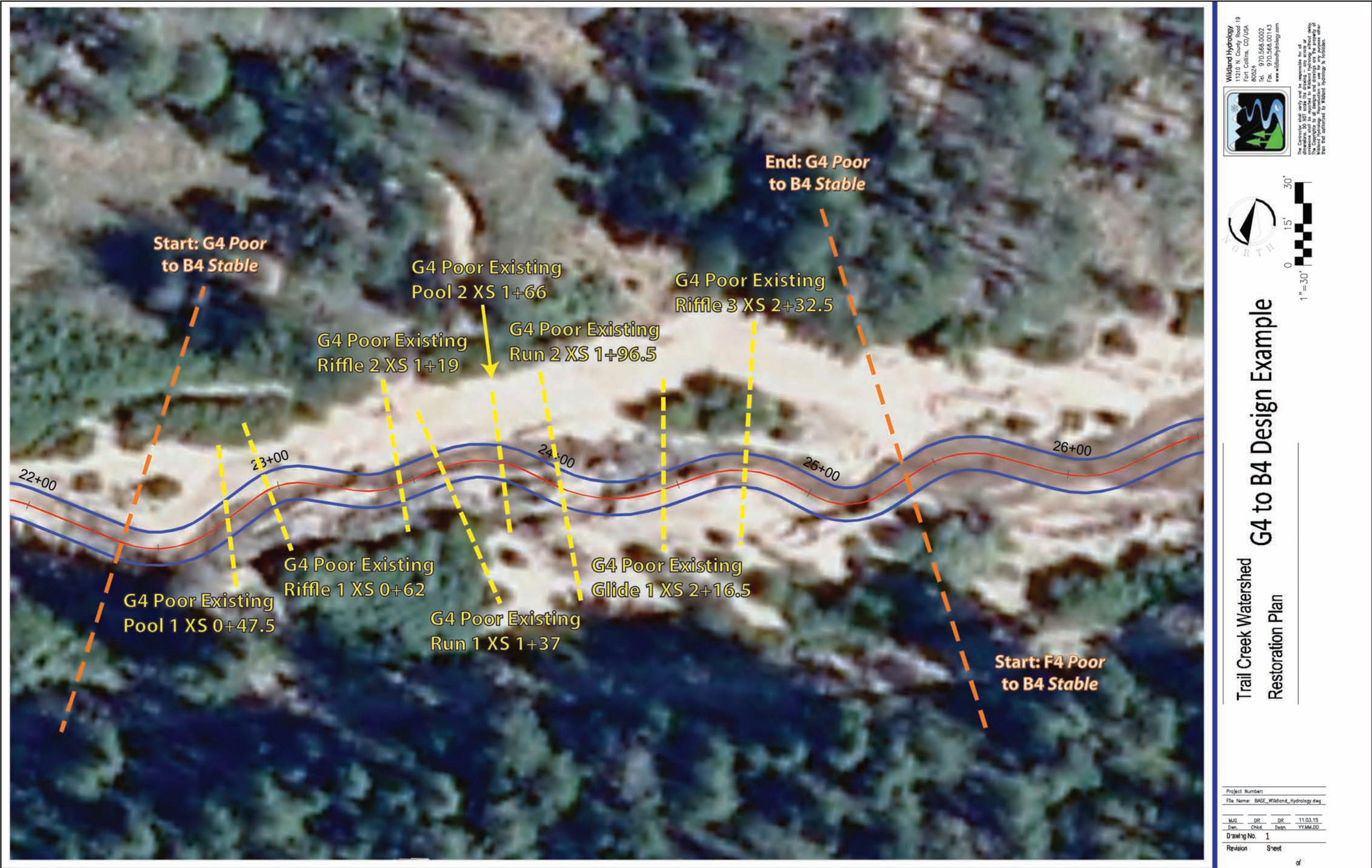
Figure 25. Plan view of the proposed conversion of the G4 to B4 stream type, including the existing G4 cross-section locations.
