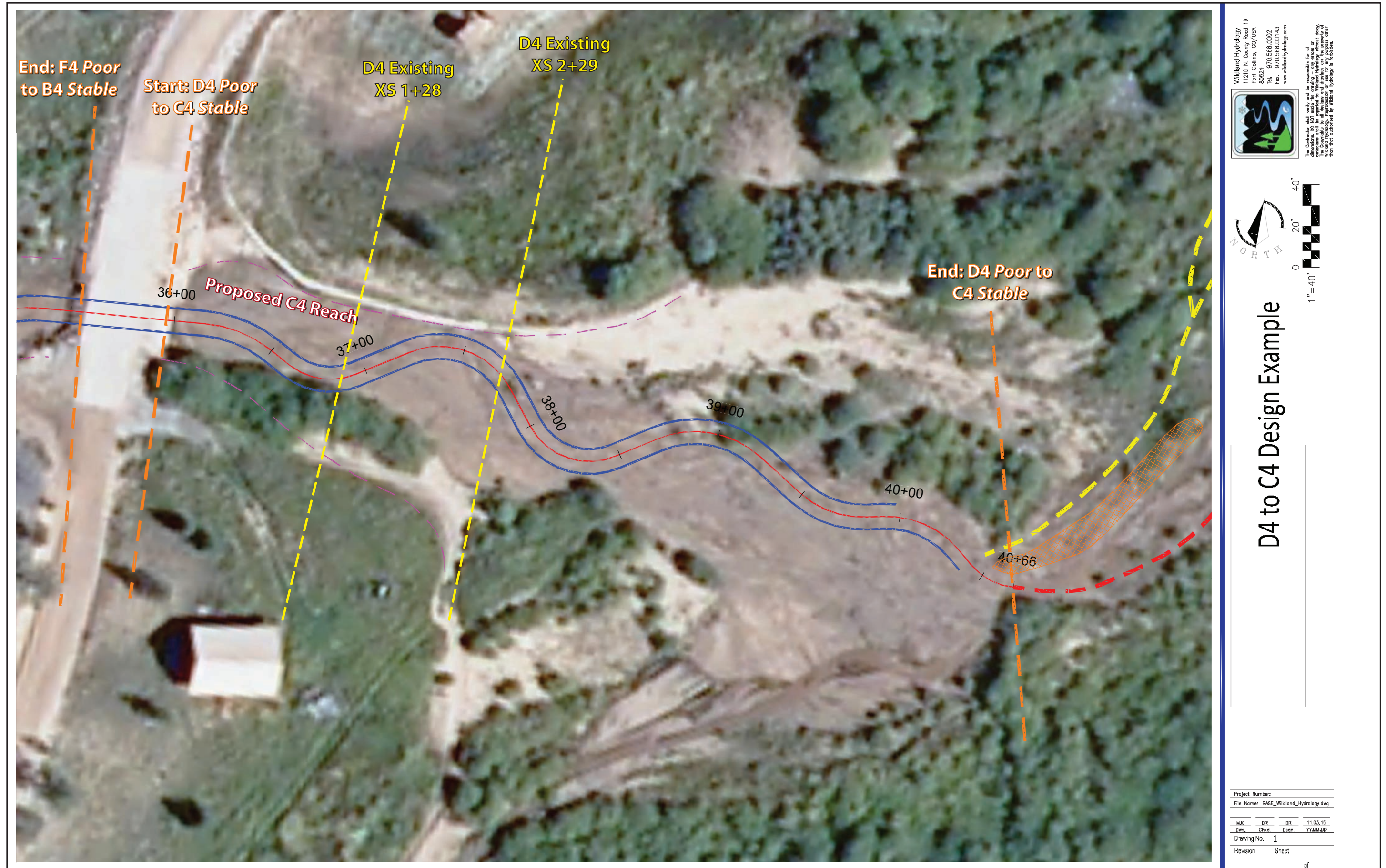
Figure 3. Plan view of the alignment for the proposed C4 stream type, including the existing cross-section locations of the D4 stream type.
