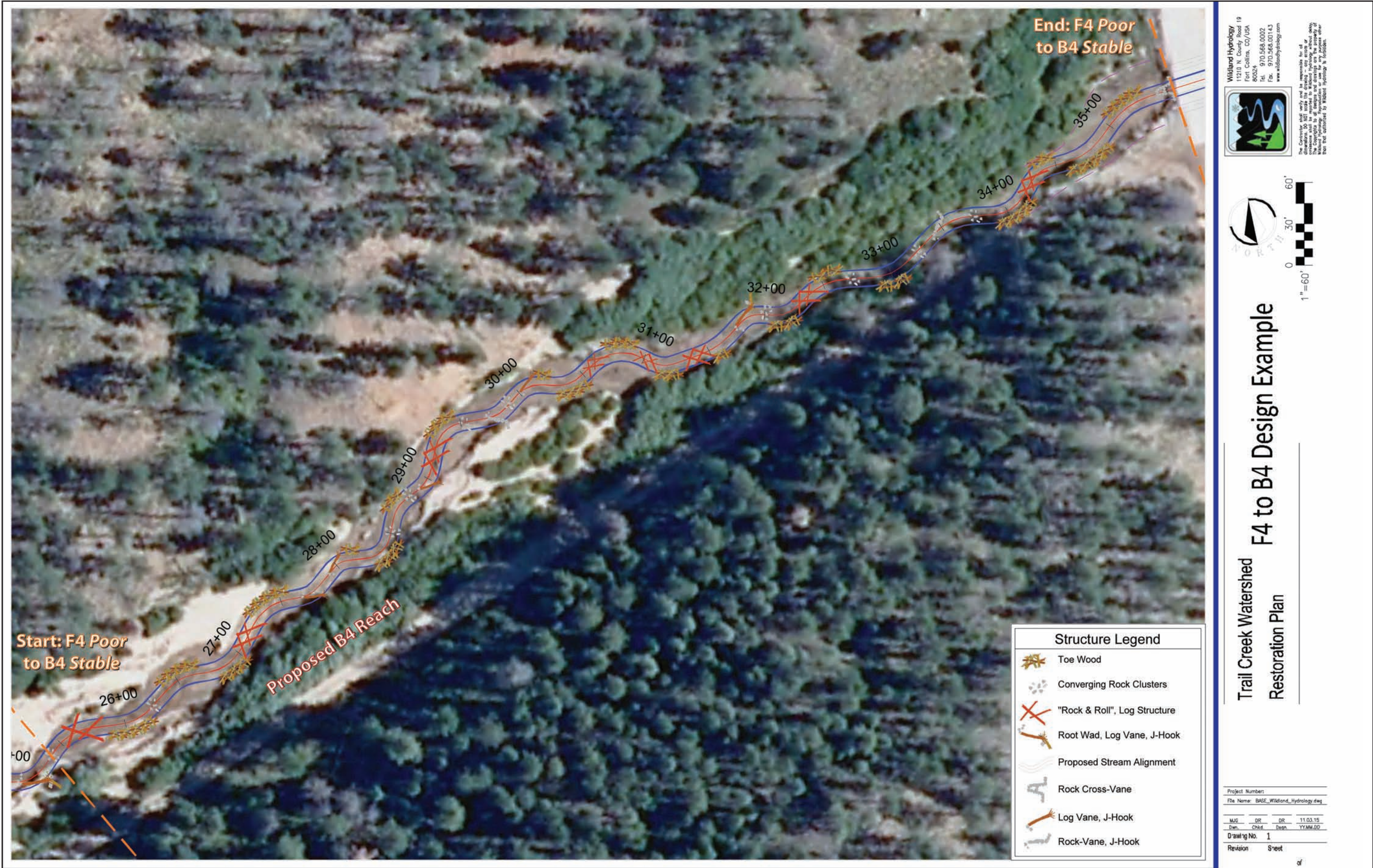
Figure 23. The proposed plan view layout of the F4 to B4 conversion depicting the stabilization and fish enhancement structures.
