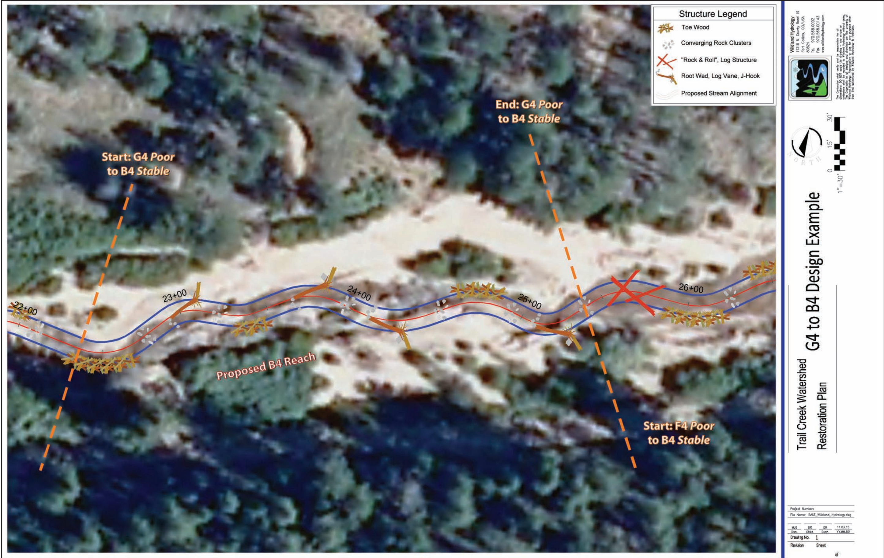
Figure 35. The proposed plan view layout of the G4 to B4 conversion depicting the stabilization and fish enhancement structures.
